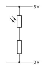
When brighter light falls on the light-dependent resistor (LDR), its resistance changes.
